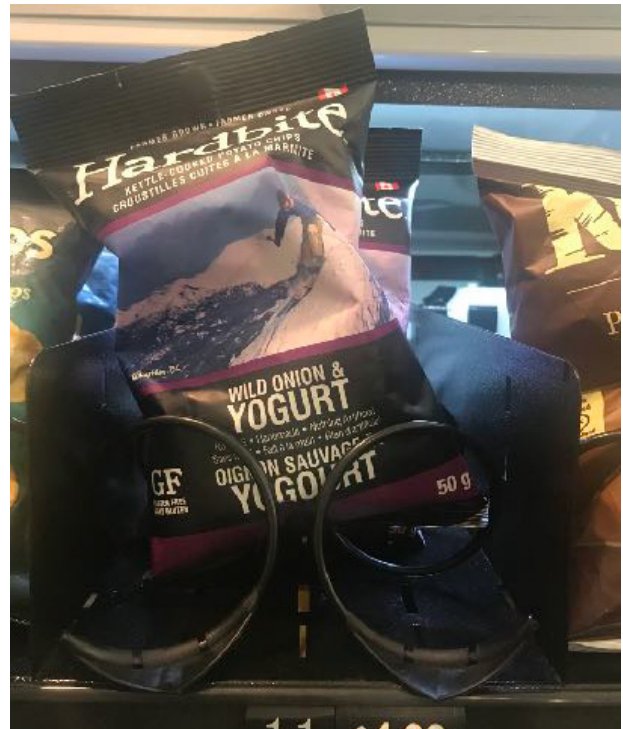
Incorrectly loaded bag product on coil
